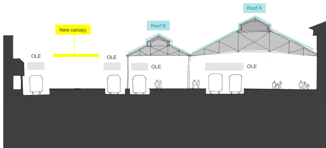
Figure 4.1.6d: Option 2 - new canopy coverage required (section)
