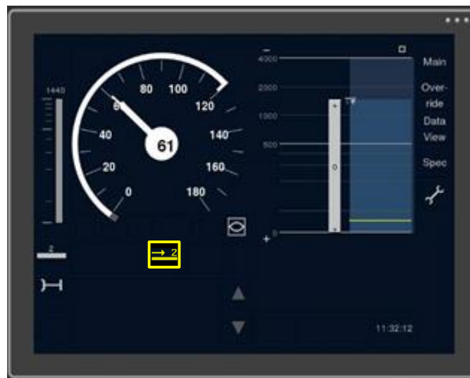
Figure 25 - Level 2 transition and acknowledgement requested
