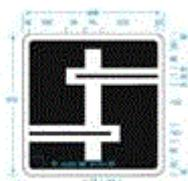
Raise pantograph at line speed
