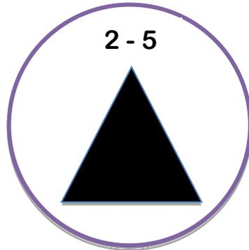
These boards are located on platforms 7 to 15, they are positioned approximately halfway along the platform and are applicable to DMUs and EMUs with a consist of 2 to 5 vehicles. The boards apply to trains travelling in either Up and Down direction, and are reversing in the station.
