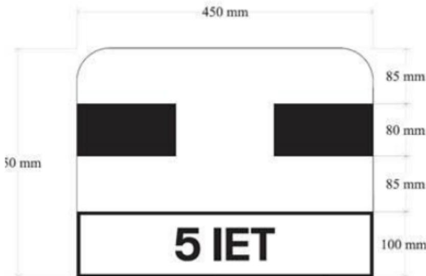
These boards are located on platforms 4, 5, 7 & 8. They are positioned halfway along the platform when travelling in the Down direction and are applicable to 5-car IETs that are scheduled to join to other services of the same traction type. Drivers of IETs not scheduled to join to other IETs must pass these signs and stop at the appropriate IET Car Stop Marker (CSM), which have been provided at the far end of each platform'.
