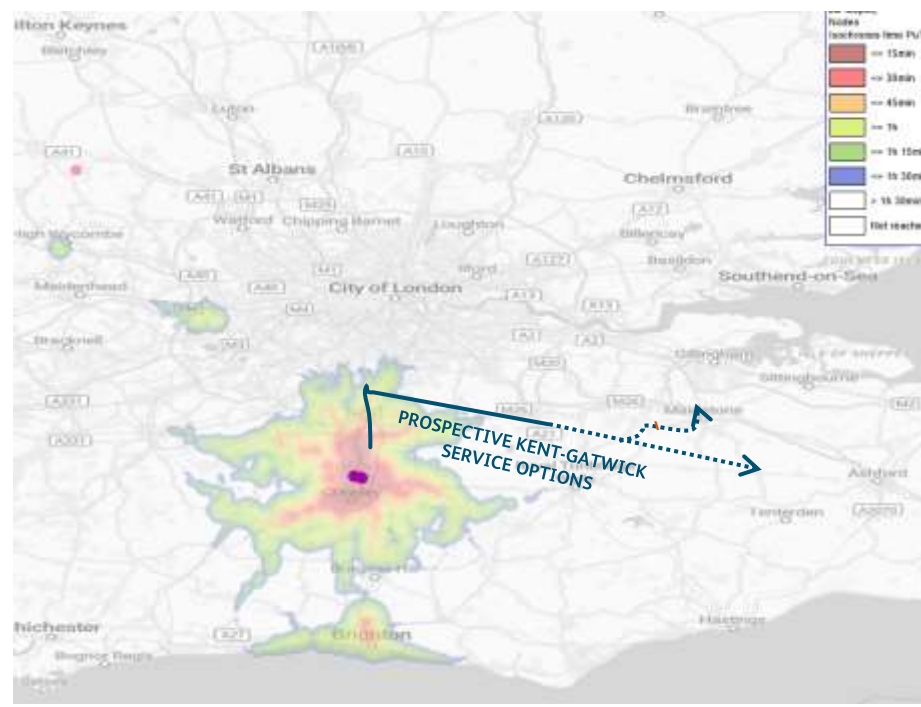
Figure 17: Bus/ Coach Journey times to Gatwick with up to two transfers. This isochrone analysis clearly demonstrates the rail opportunity for connecting Gatwick with Kent.
