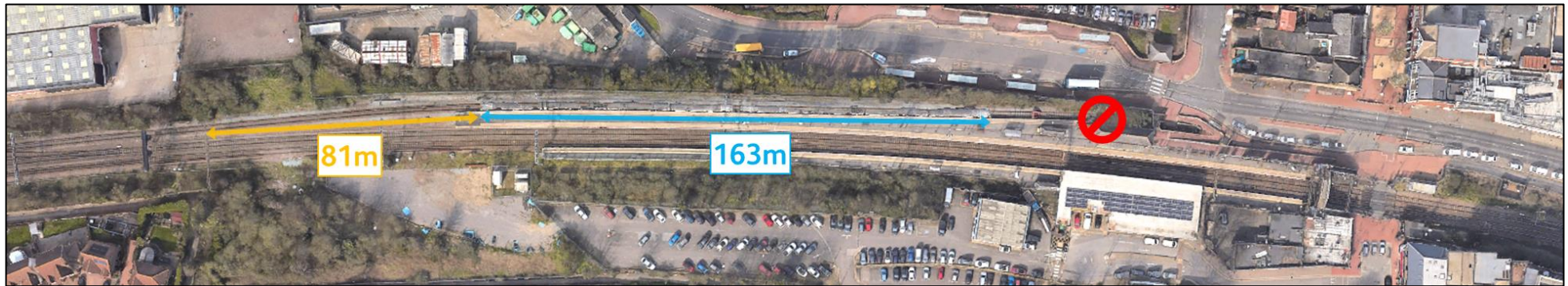
Figure 16 – Overview of Grays station and potential future platform needs, including the minimum platform extension length require, in orange.
