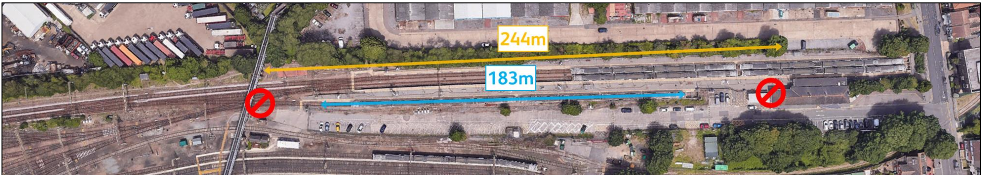
Figure 15 – Overview of Shoeburyness station and potential future platform needs. Existing shorter platform shown in blue, with potential location of future platform in orange.
