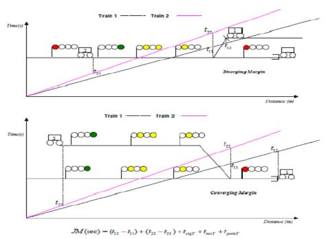
where  $t_{sigT}$  is the signal sighting time (8sec),  $t_{resT}$  is the system response time (8sec) and  $t_{poinT}$  is point movement time (8sec)
