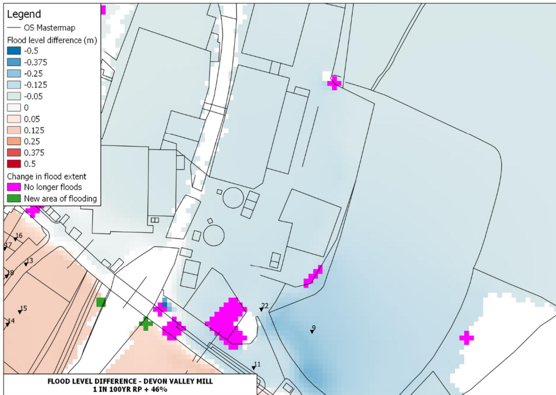
Figure 6-18 – Flood level difference between existing and proposed for 1 in 100yr+46% RP event at Devon Valley Mill
