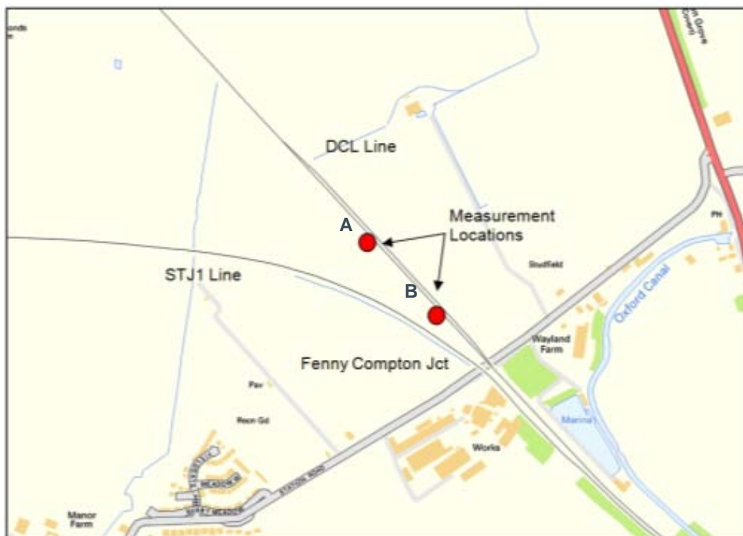
Figure 4. Vibration Monitoring Locations at Fenny Compton
