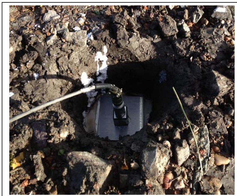
Figure 8. Example Measurement Position Accelerometer Set Up
