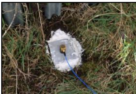
Figure 6. Example Measurement Position Accelerometer Set Up
